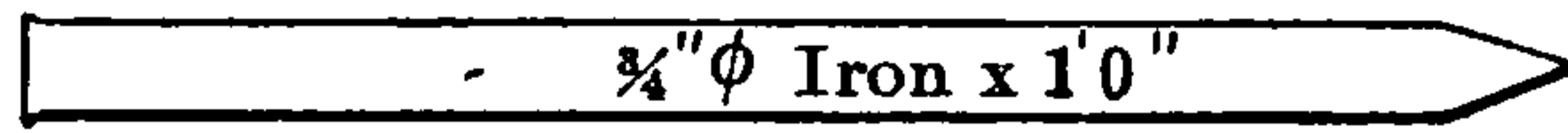
Drift Bolt, One-Half Size
